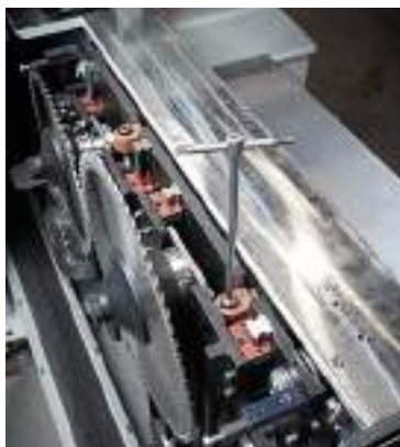
Depth grooving regulation by Sikos. Scoring regulation(left-right) from outside kit. By Sikos (optional electronic regulation with servo by PC).
